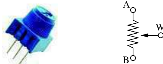
Figure 1: A typical rotary potentiometer (left). Schematic for a potentiometer (right). The middle pin is called the “wiper”.
