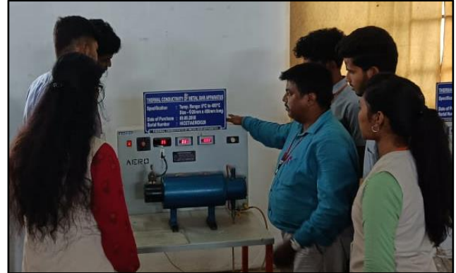
Conductive heat transfer set up
