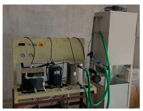
Evaporator: Shell and coil evaporator
