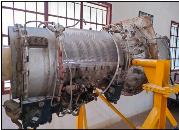
Turbo jet with visible compressor section
