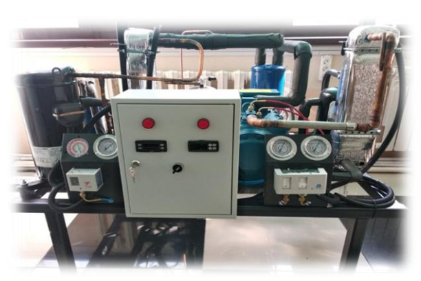
Collaborative Research project on Two stage Cascade Heat pump for space Heating
