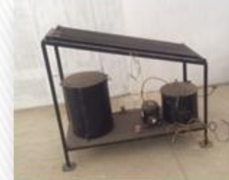
Solar Assisted Heat Pump
