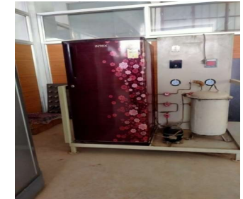
Dr. M Mohanraj Testing of domestic refrigerator using low global warming refrigerants
