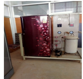
Testing of Chillers using low global warming refrigerants
