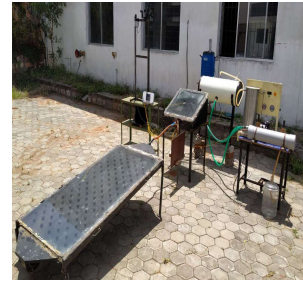
Dr. M Mohanraj Development of heat pump assisted desalination system
