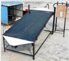
Forced Convection Solar Air Heater Using Packed Bed Absorber Plate
