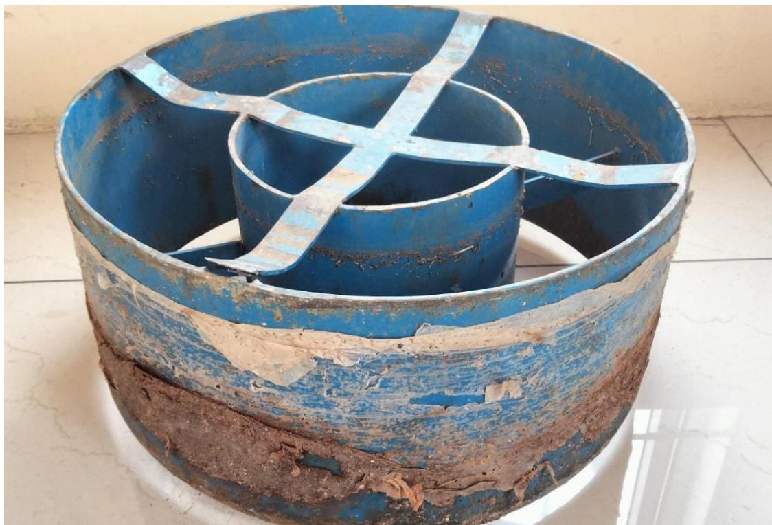
Double Ring Infiltrimeter
